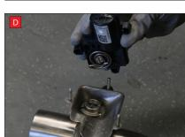
B) Lift up the motor. You will now be able to see the torsion spring (This must stay on the electronic valve motor to work with Scorpion Exhaust).
