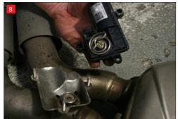
A) After you have removed O.E exhaust you will need to swap the valve motor to the Scorpion exhaust. Remove the 3 nuts ( keep safe as you will need them to bolt the electronic valve motor to Scorpion Exhaust).
